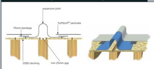
Used to form an expansion joint on roof over 50 Sqm
