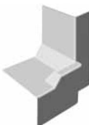
**SIMULATED LEAD FLASHING INTERNAL CORNER C7INT**
